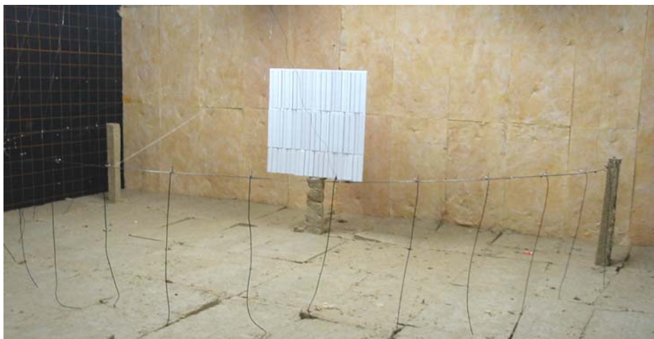
Fig. 5: Setup for the reflection measurements in an anechoic chamber
