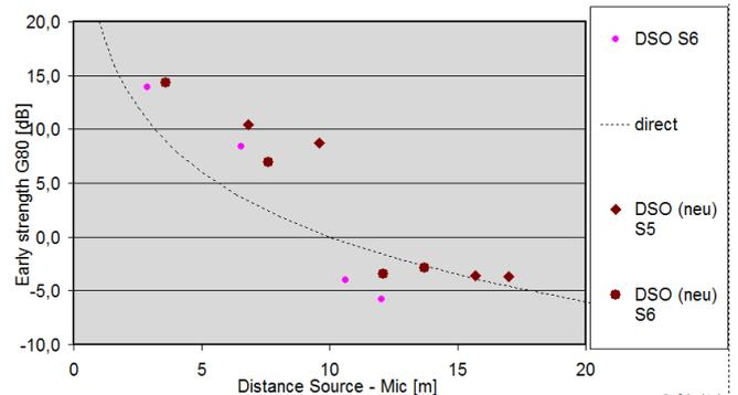
Figure 22. Measured Early Strength  $G_{80}$  before (violet) and after renovation (brown): sources in the pit and receivers on stage.
