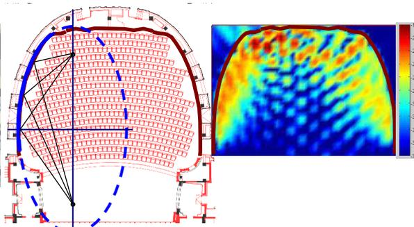
Figure 9. Floor plan of stalls (left) with the segment of an ellipse (blue) and sources and receiver points that result in focussing. Right: calculation<sup>5</sup> of the first reflection (125 Hz).
