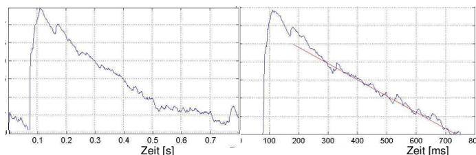
Figure 7. Measured and smoothed (20 ms) impulse response ETC from fore stage to middle of 3<sup>rd</sup> balcony of existing hall (before 2010). Left: 1:1, right: 1:10. 6 dB/div.
