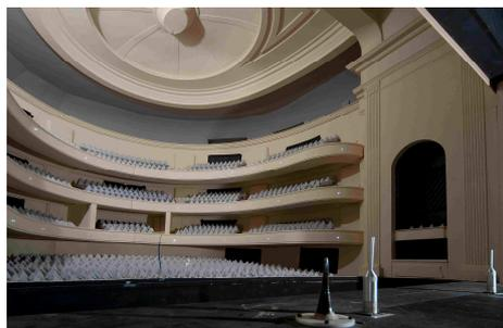
Figure 6. Scale model 1:10 with the raised ceiling and reverberation gallery. High frequency source and microphone with pre-amplifier in foreground.
