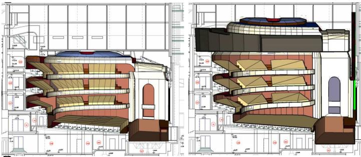
Figure 4. acoustic calculation model overlaying the longitudinal section of the hall. Left: existing before 2010, right: final design.
