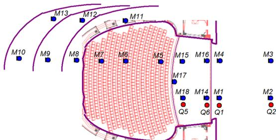
Figure 16. Sources (in red) and receivers (in blue). Balconies are schematic. Not shown: source position 7 in the pit (under Q1).
